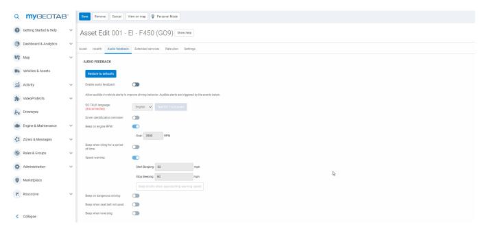
**Enable audio feedback:** When set to Off this control will override all driver feedback settings mentioned below as well as any other setting/command that would otherwise make the device beep.
